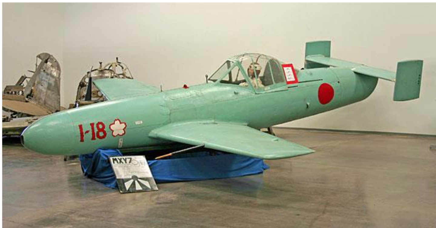
Able to reach speeds in excess of 500 miles per hour, while carrying 3000 lbs. of high explosives, the Yokosuka MXY-7 Ohka was designed to be the ultimate Kamikaze weapon.
